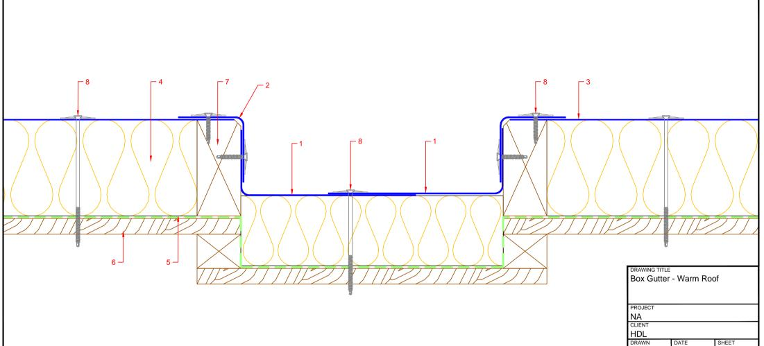
1. Dryseal trim: HDL H 0275 H 2. Dryseal trim: HDL H 0150 G 3. Dryseal flat sheet: HDL H 1250F
