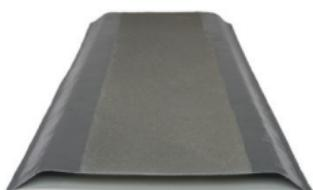
A GRP damp proof course that incorporates a wide mortar bonding strip. For use on sloping parapet walls up to 240mm thick.
