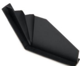
Adjustable angle stop end complete with integral bonding strip for use with most popular steel lintels to prevent the discharge of water into the cavity.
