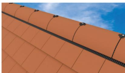
CLAY6+ is a universal ventilated dry fix ridge and hip system that can be used with all the commonly available clay and baby ridge tiles. CLAY6+ can be fitted to all roof pitches\* with no special tools required. The single unique universal jointing gasket adds flexibility and allows compatibility with the most commonly available ridge and hip tile profiles, including baby ridges.
